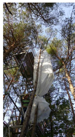
FIGURE 1 Experimental set-up of the 13 CO 2 pulse labelling of mature pine trees and the spatio-temporal 13 C tracking in stem and soil-respired CO 2 using soil collars placed at several distances in three directions from each tree stem. The 13 CO 2 addition was adjusted with a mass flow controller based on continuous 13 CO 2 measurements using a laser spectrometer. Overall 10 approximately 100-year-old pine trees were pulse-labelled, five of them growing under naturally dry conditions and five under irrigation. Adapted from Joseph et al. (2020)
